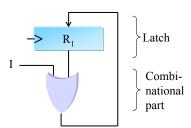
Circuits consist of combinational gates and latches (registers)
